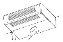
1. Securely engage the air filter in the filter guides.
