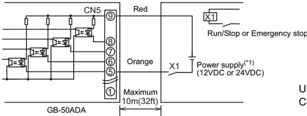
Use relays that meet the following specifications for X1, X2, Y1, and Y2.
