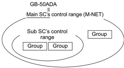
GB-50ADA is exclusively for use as a Main SC. It cannot be used as a Sub SC or controlled from a Main SC.
