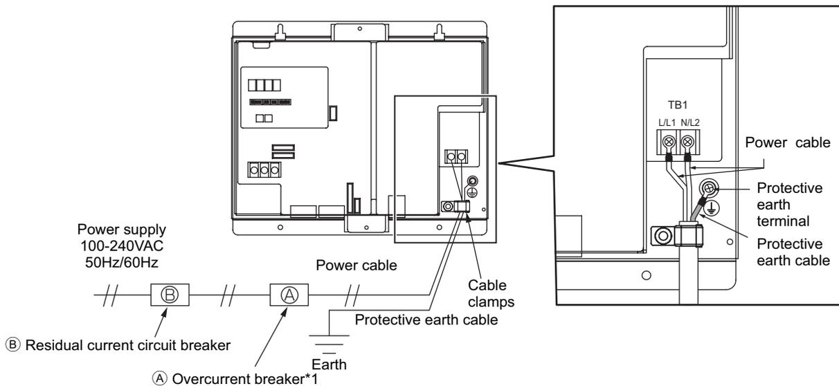
\*1 When using a fuse, use it in combination with a main switch (Rated current: 3A).
