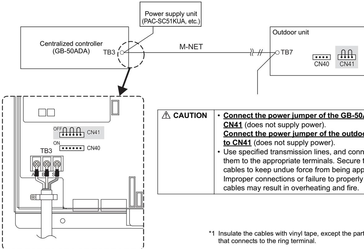
**CAUTION** • **Connect the power jumper of the GB-50ADA to CN41** (does not supply power).
