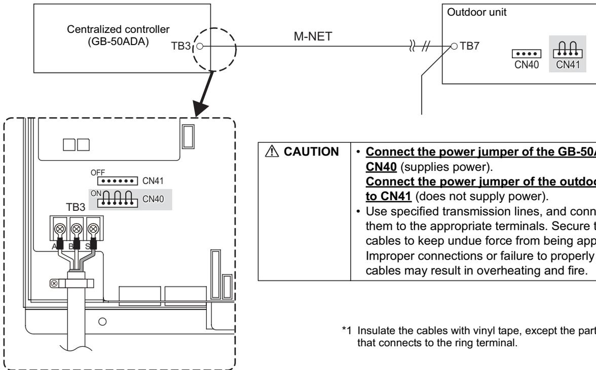
**CAUTION** • **Connect the power jumper of the GB-50ADA to CN40** (supplies power).
