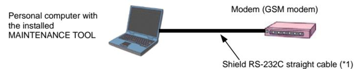
Procedure (2) After finishing the cable connection, activate the MAINTENANCE TOOL and jump to the modem setting screen. Set 3 items shown below. Refer to the [Setting procedures] on page 6. As the AT commands are used for settings, also refer to the manual of the modem.
