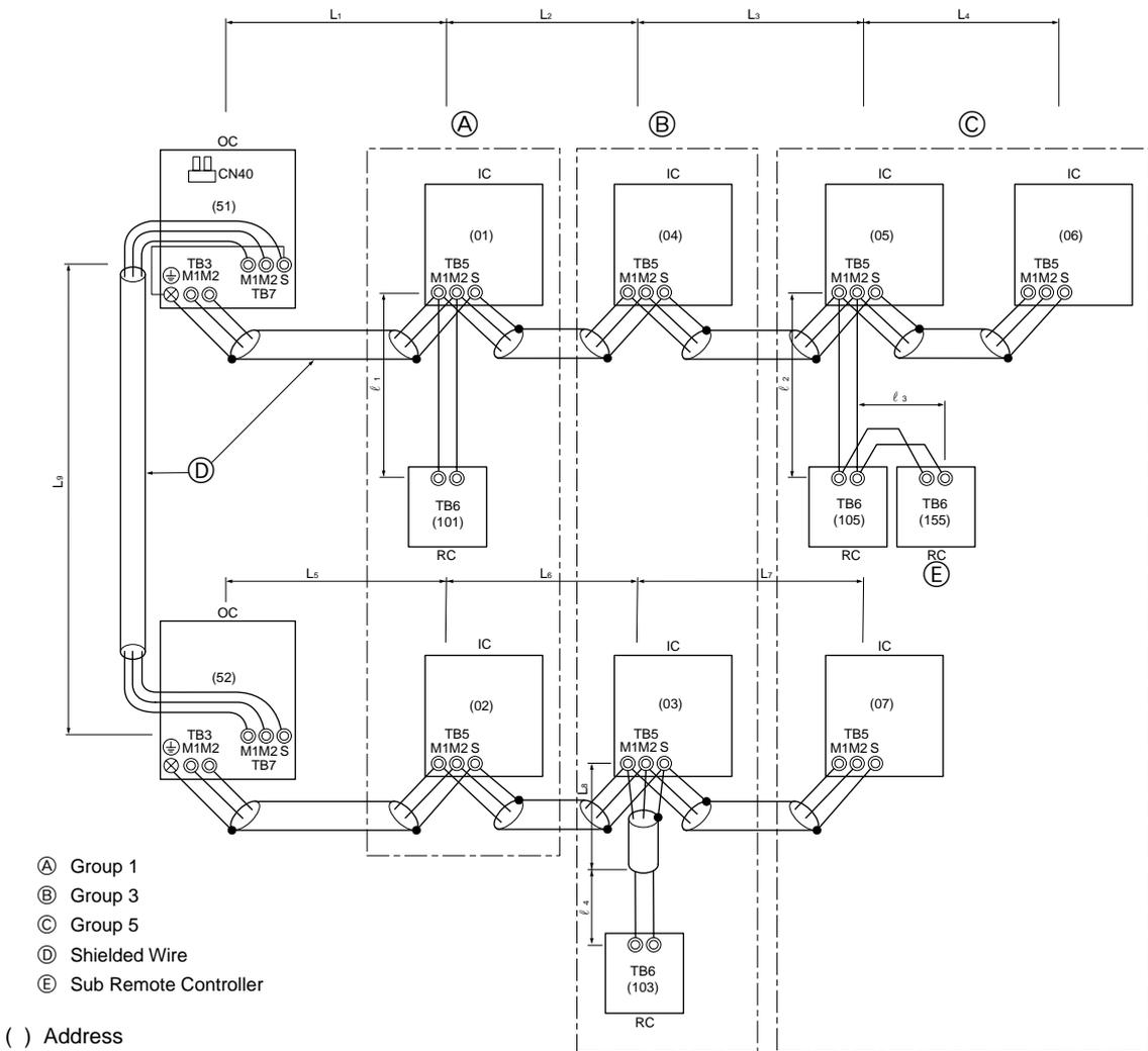
Wiring Method and Address Settings
