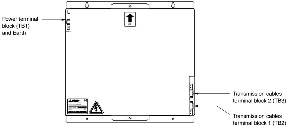
**11.3. Wiring transmission cables**
