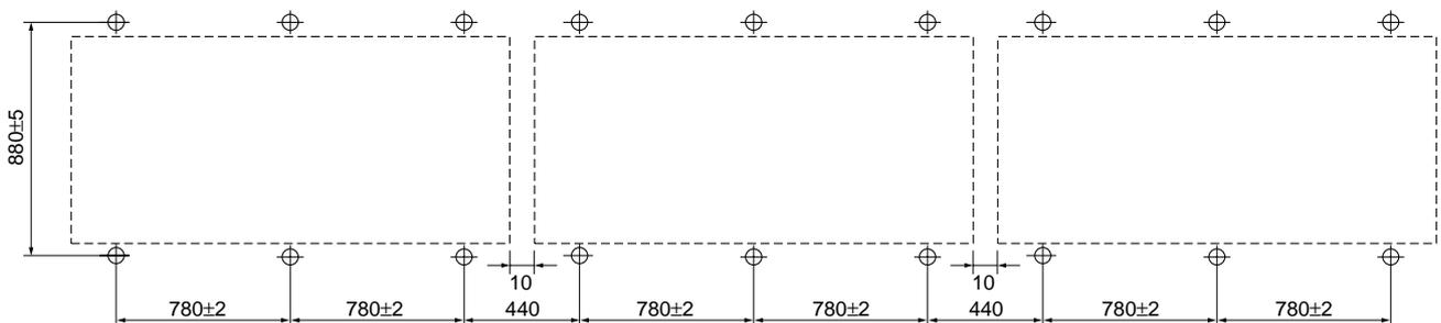
For collective installation, provide a 10 mm gap between units.
