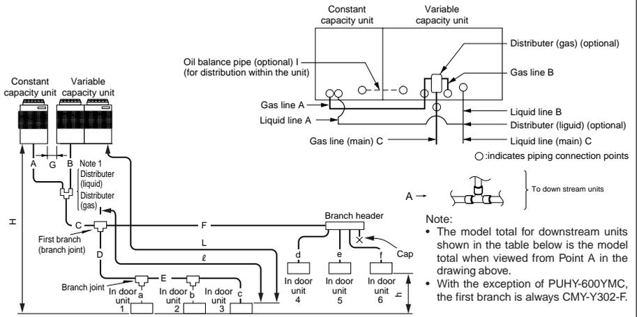
Note 1: Because it is built into the variable capacity unit, B is used to carry liquid only. Set the constant capacity unit and variable capacity unit in accordance with the G dimension given in the figure above (G = 0.01 m).
