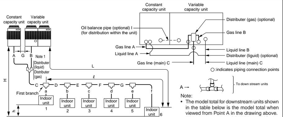
Note 1: Because it is built into the variable capacity unit, B is used to carry liquid only. Set the constant capacity unit and variable capacity unit in accordance with the G dimension given in the figure above (G = 0.01 m).
