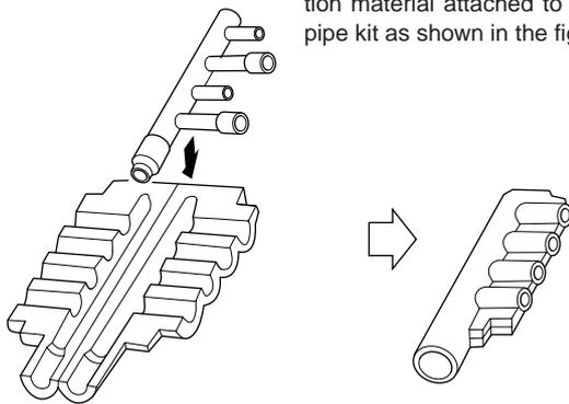
Insulate the header using the insulation material attached to the branch pipe kit as shown in the figure.
