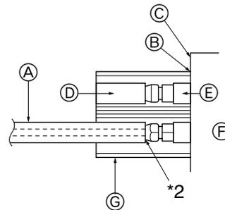
Fig-2 (figure showing the flare insulation)
