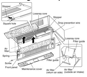
1. Securely engage the air filter in the filter guides.
