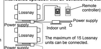
The maximum of 15 Lossnay units can be connected.
